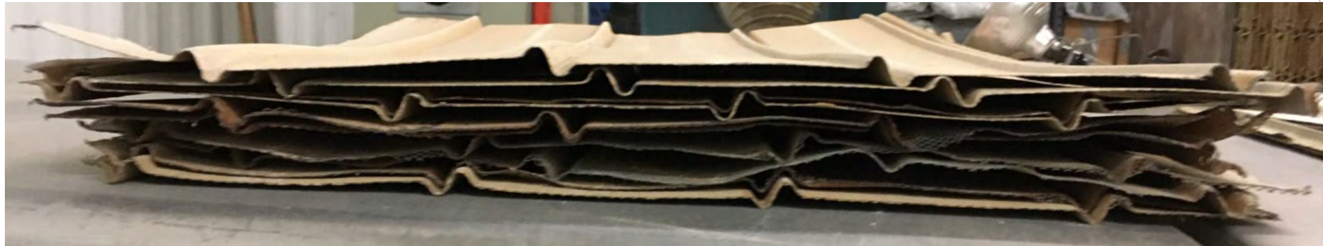
Notches Not Aligned
